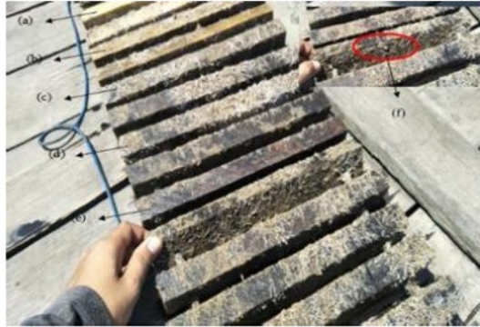
Fig. 5. Samples condition after two months bioassay (a) A. falcataria (b) V. cofassus (c) Diospyros sp. (d) D. indica (e) C. inophyllum , (f) Shells that stick to the samples
